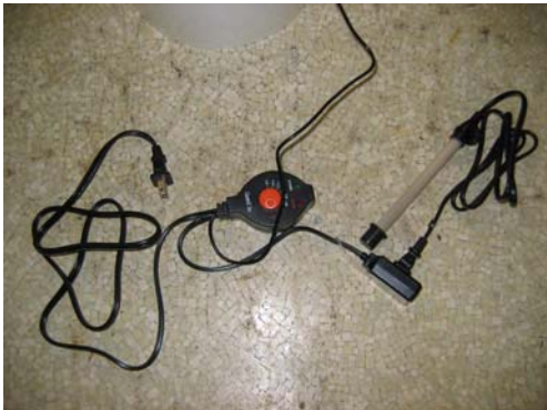
Image 1 - Thermostat Unit With Heater Attached
