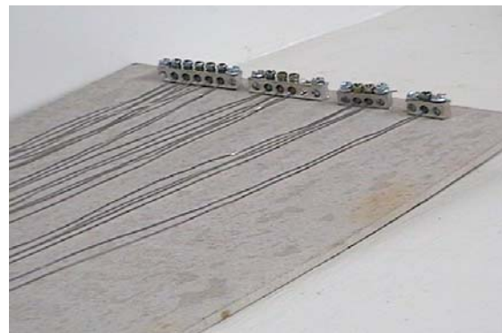
Connectors cut up and bolted to panel
