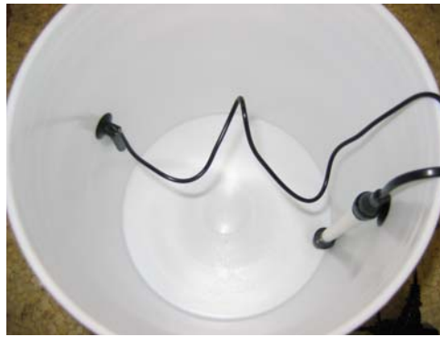
Image 2 - Heater Installed In Bucket With Temp. Sensor
